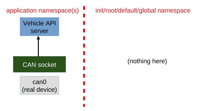
Excellent setup to run a Vehicle API which provides abstract data objects through a TCP/IP service to different namespaces via veth/IP
