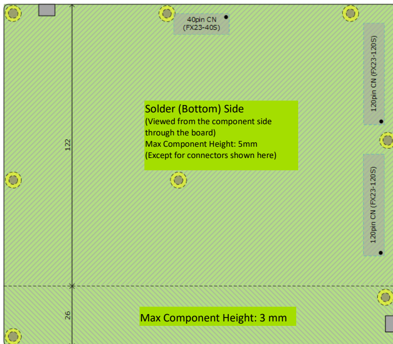
Figure 9 Vehicle/Audio Board Component Height Constraint
