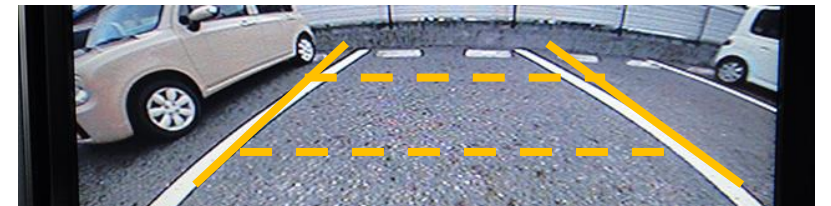
Composited rear view camera surface
